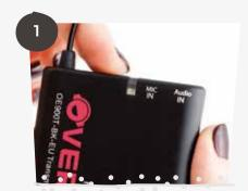
Press and hold the ON button to turn the transmitter on.
